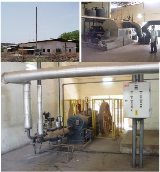
Figure 11. Sicaju plant (outside), the biomass boiler, and the steam machine
