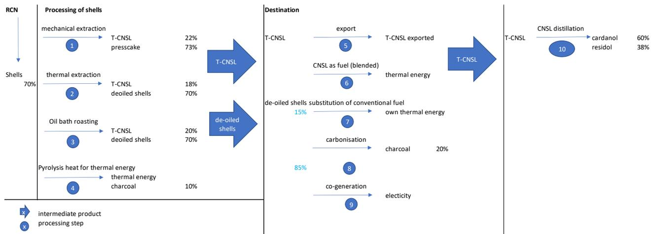
Figure 4. Flow of the main different steps in by product processing of cashew shells
